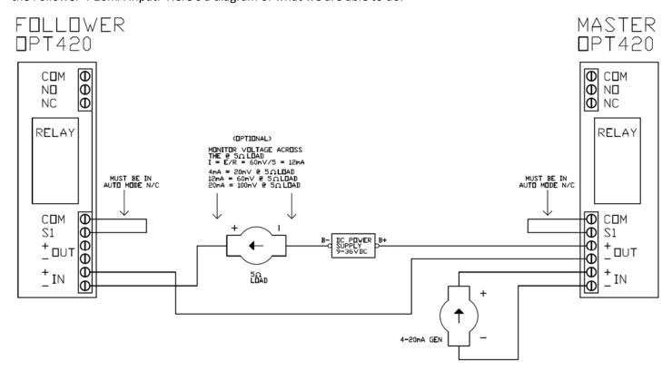
A PU Series encoder (or equivalent) is still required as the S1 input to both the Master and Follower MD/ASP device. As well, the user must supply a 9-36VDC loop power supply for the 4-20mA loop.
