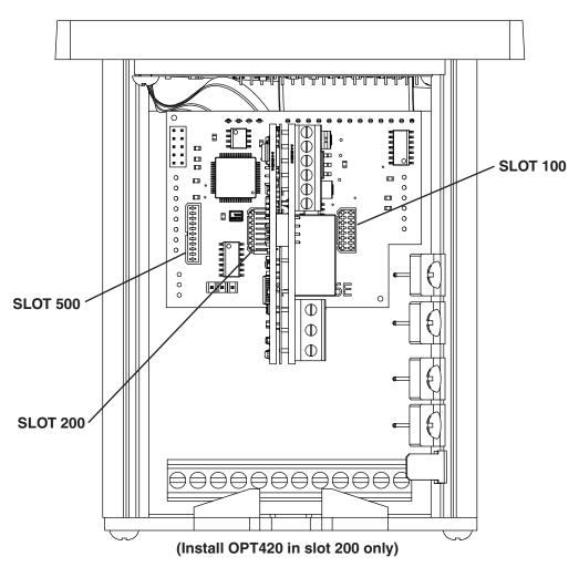
**IMPORTANT: THE OPT420 MAY ONLY BE INSTALLED IN MODULARBUS SLOT** "200". Installing in any other slot will simply result in the OPT420 "not working". Normal operation will resume when the OPT420 is placed in the Host Drive's ModularBus Slot "200".
