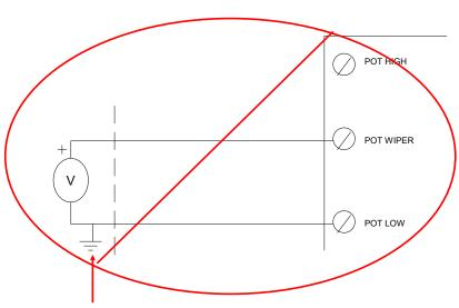
A non-isolated voltage signal input will damage the motor control electronics.
