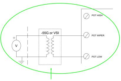
A Dart isolator board is used to protect the motor control from ground.
