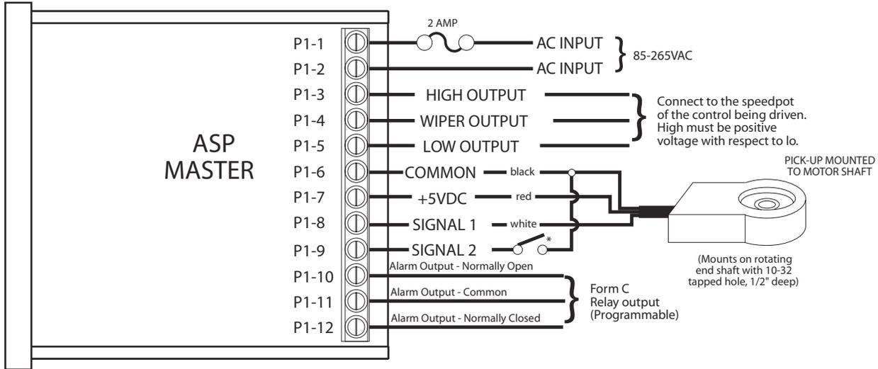
\* P1-9 signal input may be programmed for a number of functions. Incl (jog, inhibit, ect.)
