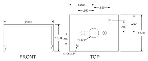
The AC03 can be secured to a panel wall via a customer supplied 3/8" Tinnerman Clip, or a self threading 3/8" nut installed over the nylon bushing of the speedpot. It may also be secured to the panel by using (2) #6 type B screws through the panel and into the .106" pilot mounting holes. Note: When using #6 type B screws to secure the control, take care to use a length that does not extend more than 1/4" through the heatsink.
