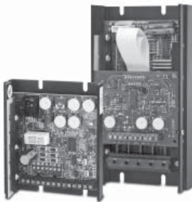
700/COMMUTROL SERIES DC BRUSHLESS 5 & 20 Amp for 12,24,& 36VDC Inputs
